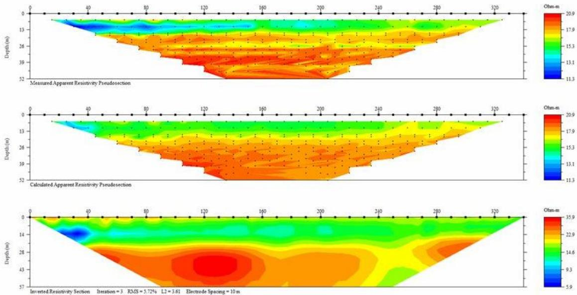
**Figure 1** – ERT apparent resistivity section and inverted resistivity section in the Baneasa area
