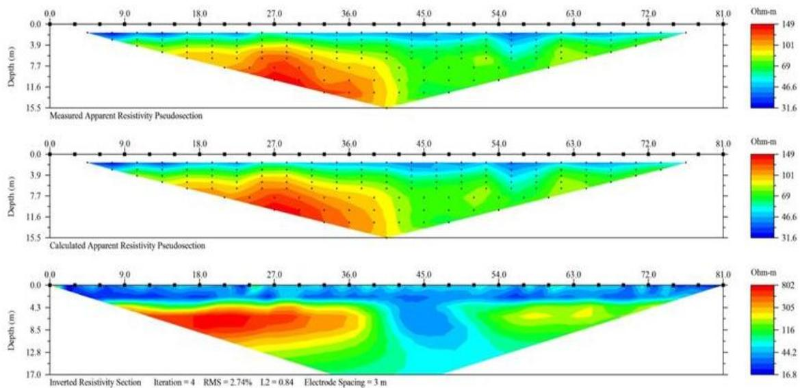
**Figure 2** – ERT apparent resistivity section and inverted resistivity section in the northern part of Bucharest
