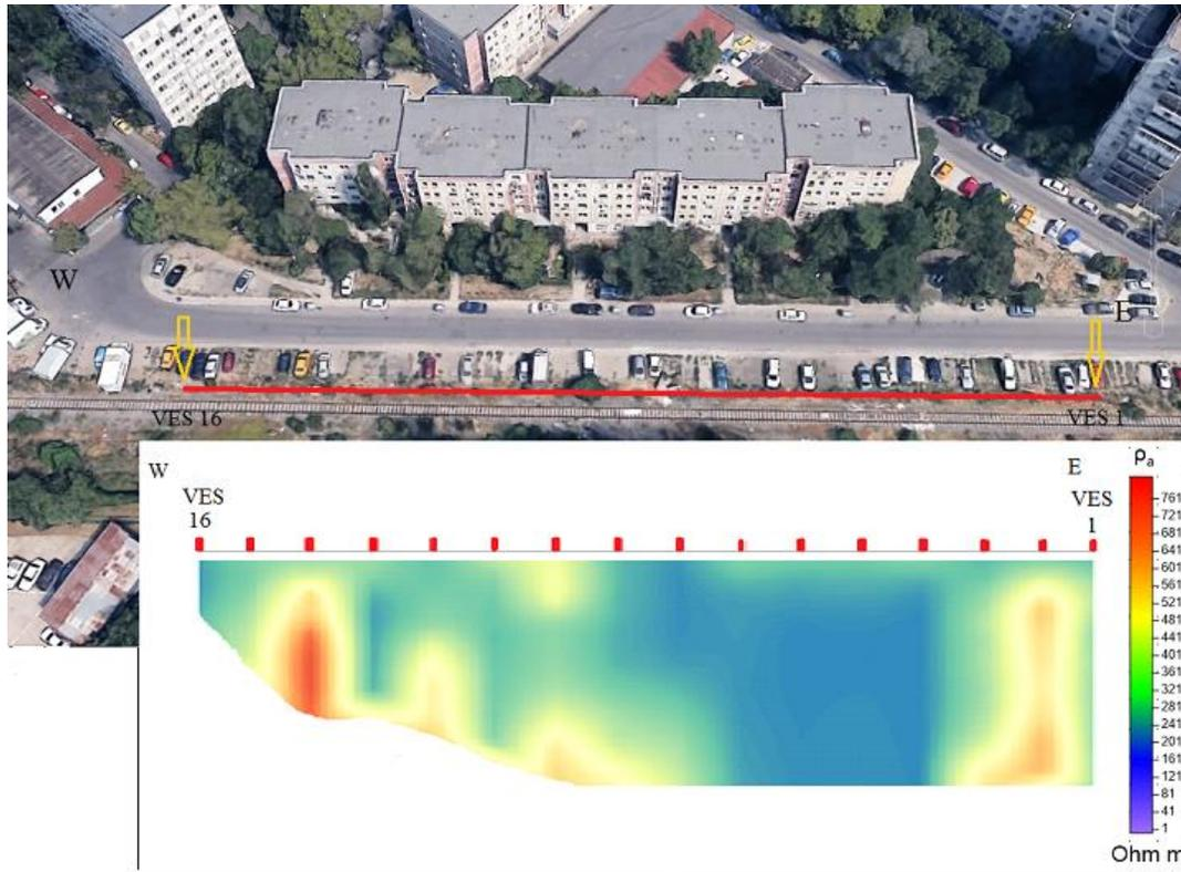
**Figure 3** – VES resistivity data (50m depth) in the western part of Bucharest
