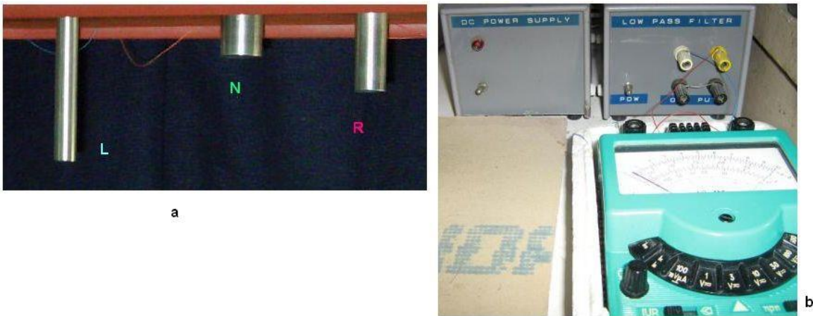
Fig. 1 a) brass cylinders of electrodes: L - left, R - right and N - null; b) low pass filter (ULF) and the analog multimeter
