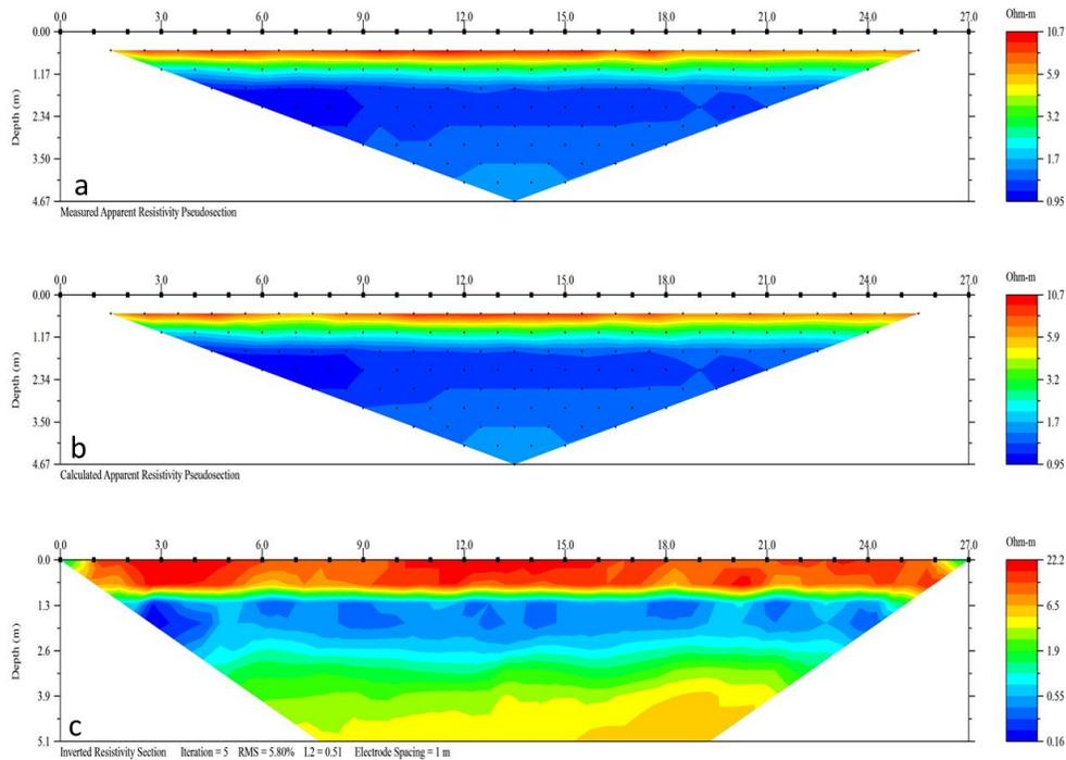
**Figure 1** – Electrical resistivity tomography section obtained using Wenner array a) Measured apparent resistivity data, b) Calculated apparent resistivity data, c) Inverted resistivity section
