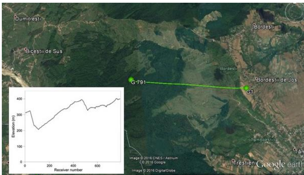
Figure 2: Topographic map for the Dumitresti area, Romania, showing the seismic line (green line); inset: elevation variations along the line. Source map: http://maps.google.com .
